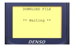
2) Transfer the new program (PD3 or PD4) file from the PC by running the Winartu3 shortcut (or selecting send on the Program Loader). The display will show the transfer progress and BEEP twice when completed. Now press **C C** to return to the SYSTEM MENU.
