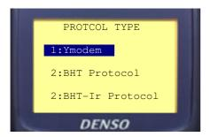
**Important** Once the new program has been loaded, the protocol must be set back to **BHT PROTOCOL** in order for the day to day data transfers to work correctly.
